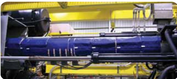
QuickCool fully enclosed to increase energy efficiency during high-temperature process job.
